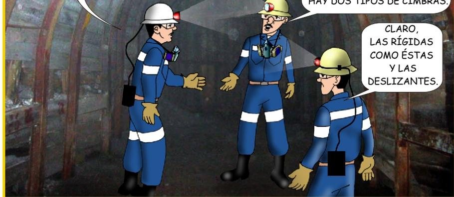
LAS CIMBRAS RÍGIDAS USAN COMÚNMENTE PERFILES COMO LA "W", "H" E "I", CONFORMADAS POR DOS O TRES SEGMENTOS UNIDOS POR PLATINAS Y PERNOS CON TUERCA.
