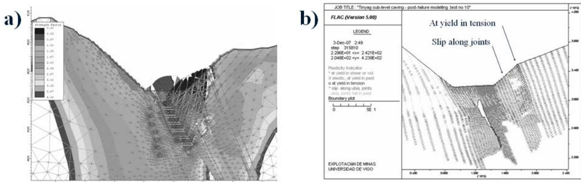
**Figure 8** Longitudinal numerical modelling of Tinyag: a) Phase-2D detail model in 8 stages of mining, substituting ore by caved and fractured material and b) Flac-2D simulation of the process of caving where the main instability mechanisms are identified, a further refinement of the model is needed to interpret it in a quantitative way.
