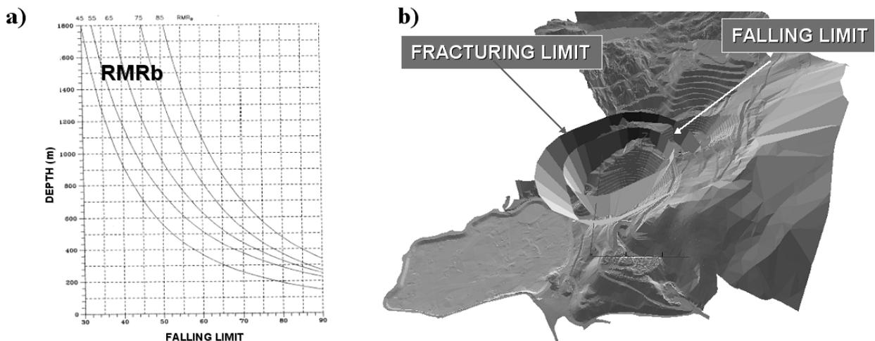
**Figure 6** a) Estimate of the falling angle limit as developed by Chilean researchers and b) estimate of falling and fracturing affection for the case of Tinyag SLC.
