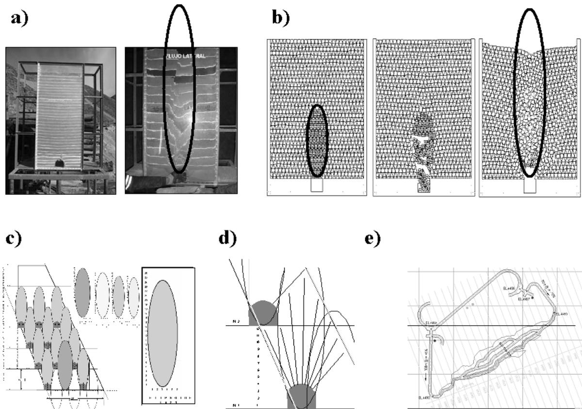
**Figure 4** a) Physical modelling of the extraction and loosening ellipsoids for Rosaura mine. b) UDEC verification of the extraction ellipsoid for Tinyag. c) Estimate of the extraction ellipsoid for the thicker part of Tinyag for longitudinal SLC. d) Drill ring scheme in a narrow zone of Tinyag seam e) Plan view of the longitudinal SLC design for Tinyag in an particular level.
