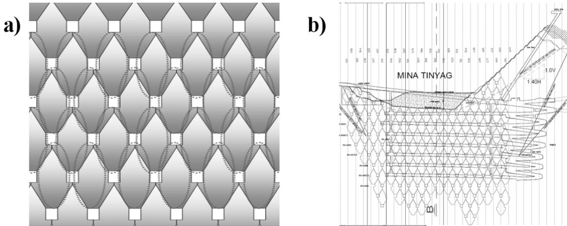
**Figure 5** a) Basic “improved” SLC design for Tinyag mine and following Bull and Page (2000) and b) General view of the mine design for Tinyag transversal SLC.
